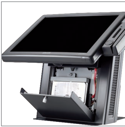
TOOL FREE ACCESS TO HARD DISK
